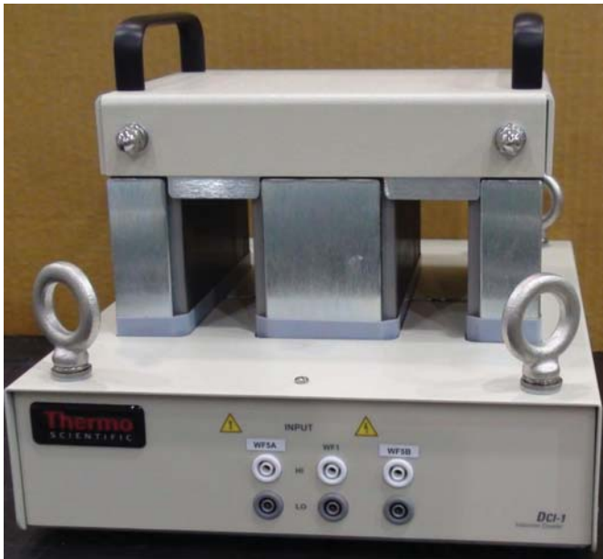
Figure 12 – Injection Transformer For Waveforms 1, 5A and 5B
