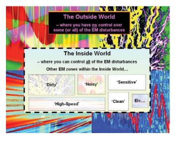
Figure 5A Segregating circuits into Inside and Outside worlds
