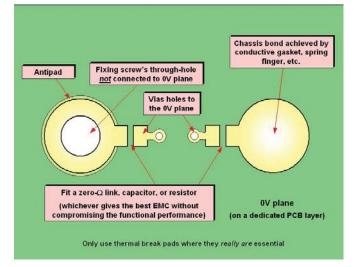
Figure 5H Example flexible 0V plane – chassis bond layout
