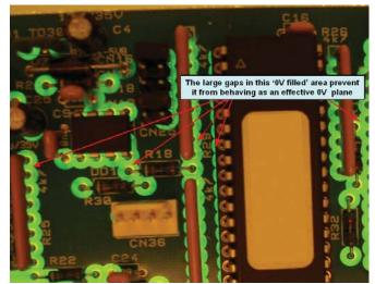
Figure 5F An example of how not to design a plane.
