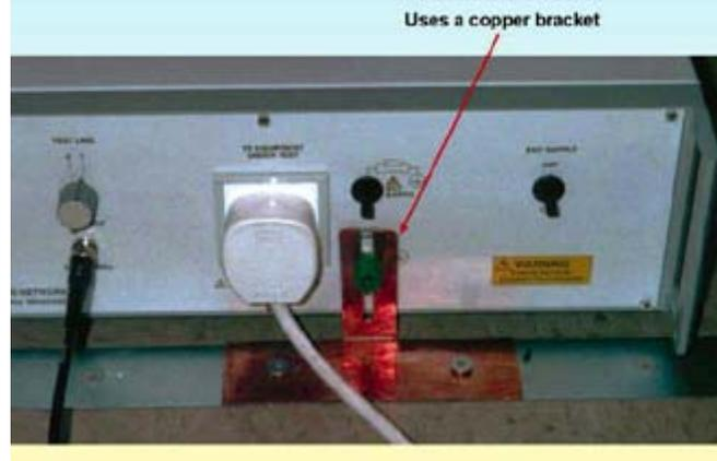
Perfectly good LISNs can be purchased for around £600 (UK Pounds), but if you wish to construct your own you should recognise that constructing an accurate LISN is not as simple as its schematic. Here are a few essential construction tips extracted from [3] and [4]:
